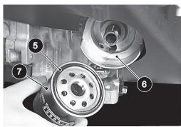
The oil capacity is 1-1/3 quarts (1.3 liters). Add slightly less than 1-1/3 quarts (1.3 liters) to allow for possible residual oil left in the engine. The oil must be high quality and meet or exceed API SF, SG, CC standards. Check the oil level on the dipstick. Oil should be slightly below H to allow for expansion. If necessary, continue to add oil slowly and allow time for the oil to flow down into the engine. Check the oil level on the dipstick. **Do not overfill**.
