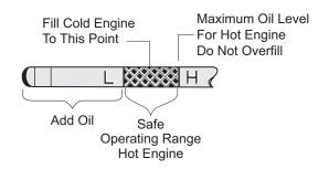
The oil dipstick/fill cap must be in place before operating the engine. Failure to install the dipstick/fill cap will result in oil becoming contaminated and/or oil being discharged into the engine compartment.
