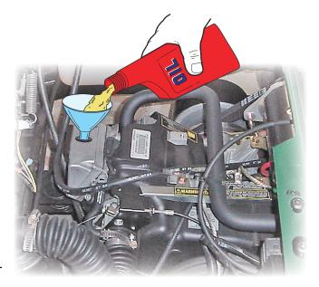
Start the vehicle. Allow the engine to run for a few minutes to fill up the oil filter. Stop the vehicle on a level surface, set the parking brake and remove the key. Check for oil leaks at the drain plug and oil filter. Tighten the drain plug or oil filter if a leak is found. Check the oil level on the dipstick. Add oil if necessary.
