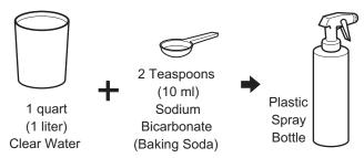
The correct cleaning method is to spray the top and sides of the battery with a solution of baking soda and water. Apply this solution with a plastic spray bottle. The solution is 2 teaspoons (10 ml) sodium bicarbonate (baking soda) mixed with 1 quart (1 liter) of water. Spray the solution on all metal components near the battery also.
