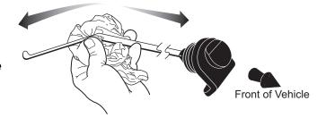
The oil should be checked with the engine warm. The vehicle should be on a level surface with the parking brake engaged. Allow adequate time for oil to drain into the crankcase before checking.
