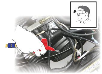
At least once a year, (or more often under adverse conditions) the cooling system should be cleaned. Cleaning will assure an adequate supply of air to the cooling fins. Compressed air may be used for routine cooling system maintenance.
