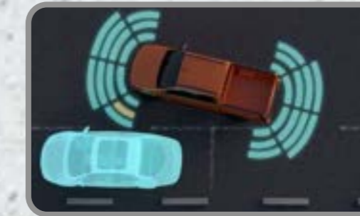
FRONT AND REAR PARKING SENSORS: Sensors provide feedback on nearby obstacles when parking in tricky spots.
