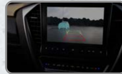
REVERSE CAMERA: Your ISUZU D-MAX ARCTIC TRUCKS AT35 triggers audio and visual warnings should anything approach from left or right while you are reversing into traffic.
