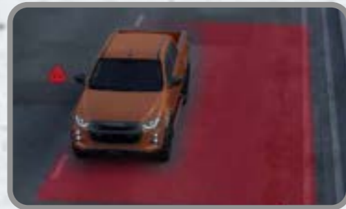
LANE KEEP ASSIST (LKA): Should your ISUZU D-MAX ARCTIC TRUCKS AT35 start to move out of its lane, Lane Keep Assist (LKA), Emergency Lane Keeping (ELK) and Lane Departure Prevention (LDP) help to correct this and prevent collisions.
