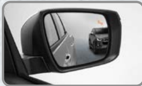
BLIND SPOT MONITOR [BSM]: Your ISUZU D-MAX ARCTIC TRUCKS AT35 displays a visual warning in your side mirrors when a vehicle approaches in your blind spot.
