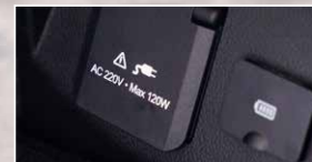
120 WATT 220V INTERIOR POWER OUTLET.
