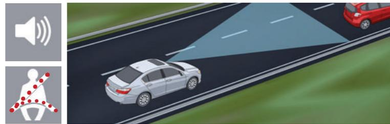
Secondary warning: If the distance between the two vehicles continues to decrease, CMBS® applies light braking and the seatbelt E-pretensioners in the driver's side gently pull two or three times. At this point the E-pretensioners pull the seatbelts with enough force to properly restrain you and your front passenger, giving you time to react and avoid a collision.
