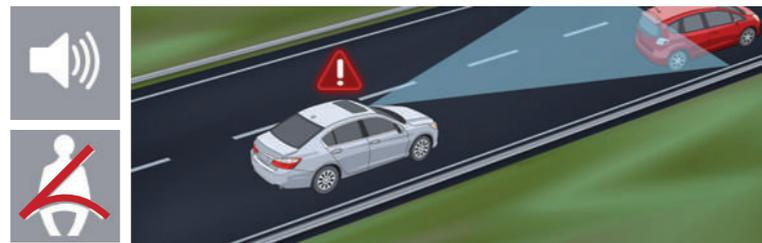
Third warning: At this stage, there's a chance that a collision will occur. The CMBS® system starts emergency braking and activates the brake assist function to reduce speed. At the same time the seatbelt tightens to reduce the impact of the collision on the driver and front passenger.
