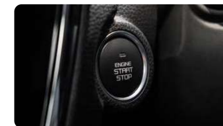
Passive entry/start system with engine push start/stop button and remote start engine.**
