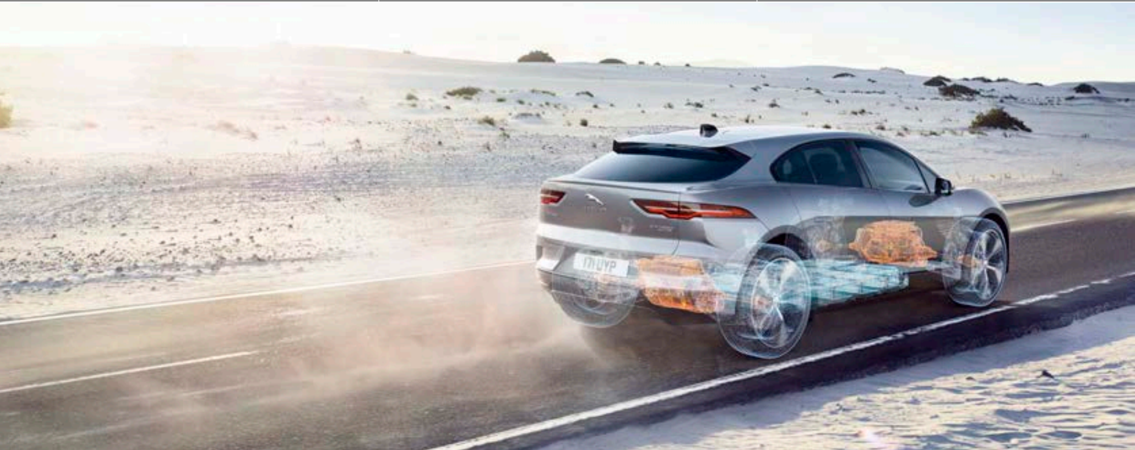
■ Battery Pack ■ Electric Motors
