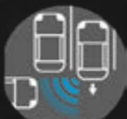
**Rear Cross Traffic Alert** Backing out of your parking space, Rear Cross Traffic Alert monitors the rear of your Navara and warns you about cars it detects creeping up from either side.
