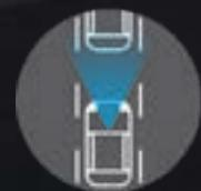
**Intelligent Emergency Braking** Help if you need it. It monitors your speed and distance between you and the car ahead and can let you know if you need to slow down. It can also automatically engage the brakes to help avoid a collision or lessen the severity of an impact.
